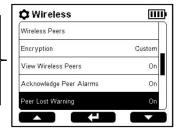
The navigation bar provides control symbols. Each action displayed in the navigation bar is controlled by the button underneath it. The action on the left is controlled by the left button ( $\blacksquare$ ), the action shown in the center by the power button (4), and the action shown on the right by the right button ( $\blacksquare$ ).
