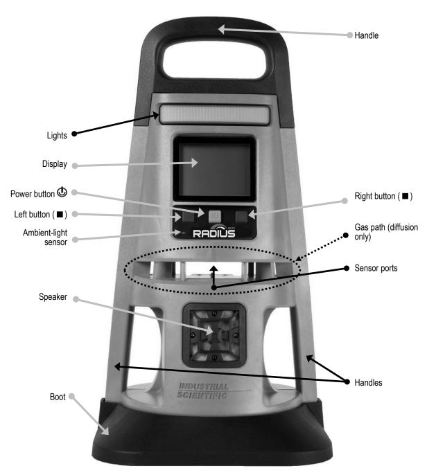
Figure 3.1.A Hardware overview Radius BZ1 (front view; diffusion)
