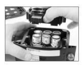
Hold the sensor collar by the edges. Lift it straight up to remove it; set aside the collar for later reassembly.
