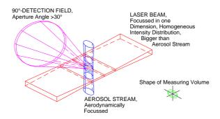
Schematic view of 90° measuring arrangement
