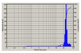
Primary measuring result for a 26.15  $\mu m$  polystyrene latex (PSL) aerosol
