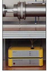
Fractional collection efficiency of oil mist separators, determined by means of a Topas Separator Performance Tester SPT 140 Straightforward investigation of the fractional collection efficiency in dependence on the load in the raw gas (setup including a SYS 520 switching unit below a Topas filter testing channel AFC 131)
