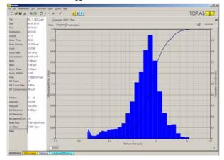
Oil droplet size distribution measured at 80°C, 4 bar nozzle pressure within Topas oil mist separator test rig SPT 140.
