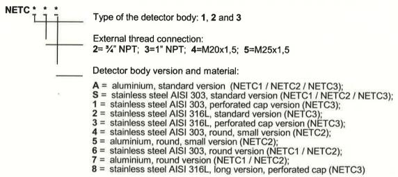
The types NETC6, NETC7 and NETC8 are characterized by the presence of a sealed glass in place of the sintered element. Within these models of the detector are present electronic circuits that use the principle of the optical radiation (infrared or laser) to measure the concentration of the gas detected. These circuits comply with IEC 60079-28 standard and the detectors have a combined type of protection: "Ex-db" flameproof associated with "Ex-op is" inherently safe optical radiation.
