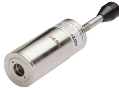
IR-CAST 2C is a highly accurate digital two colour Rectangular measuring field IR pyrometer for non contact temperature measurement specially used in foundries for molten metal. The Pyrometer measures the temperature of an object by calculating the ratio of the energies at two different wavelength bands. The ratio technique eliminates and reduces errors in temperature measurement caused by factors such as dust, vapour or smoke etc.
