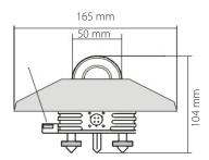
LPPYRA02 is also available in the version with shadow-ring (LPPYRA12) This measures the diffuse solar radiation eliminating the contribution of direct irradiance.
