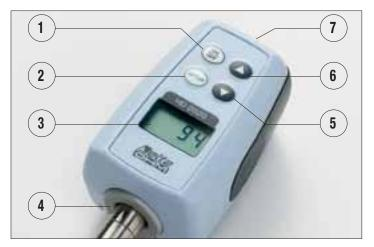
The clock/calendar allows you to set the number of years and months of validity of the calibration from the date of adjusting: at the expiration time, an appropriate symbol flashes on the display.
