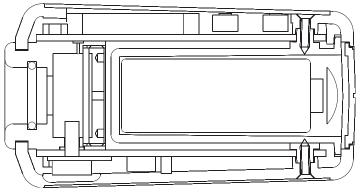
Fig. 3 Mechanical construction of the calibrator (section).
