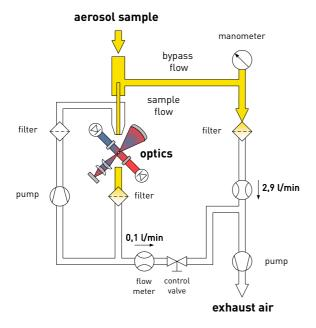
Principle of operation of the laser aerosol particle size spectrometer LAP 325.
