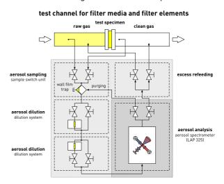
Principle of operation of the fractional efficiency measurement system FMS 375.
