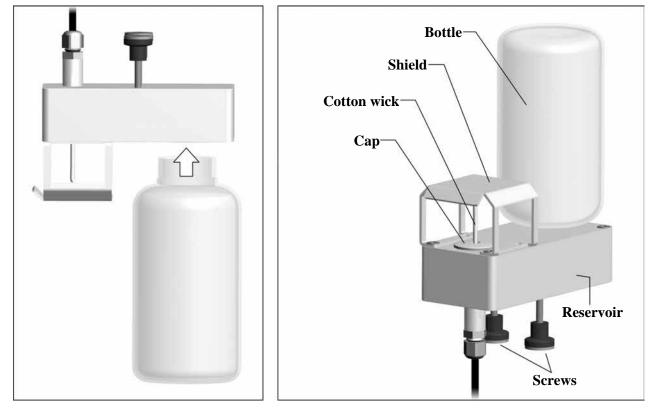
For measurements in presence of solar irradiation, use the protection shield from solar radiations. The cotton wick calcifies (becomes hard) with time: replace it periodically.
